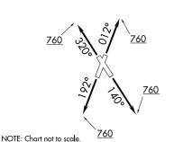
TAKEOFF RUNWAY 14: Climb on heading 140° to 760 for RADAR vectors to KNTKY, thence. . . . TAKEOFF RUNWAY 19: Climb on heading 192° to 760 for RADAR vectors to KNTKY, thence. . . . TAKEOFF RUNWAY 32: Climb on heading 320° to 760 for RADAR vectors to KNTKY, thence. . . .
