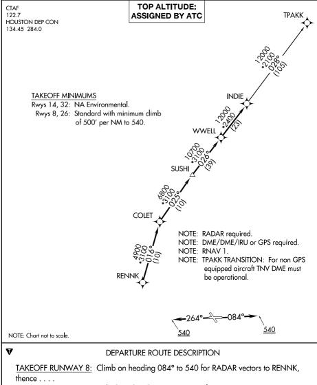
TAKEOFF RUNWAY 26: Climb on heading 264° to 540 for RADAR vectors to RENNK, thence . . . .
